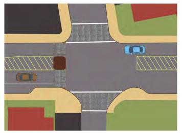
Pictured above is a concept plan for the mid block crossing at Central Ave on Huntingdon Pike. Existing conditions are shown in the photograph to the right and a photosimulation below depicts the proposed improvements.
